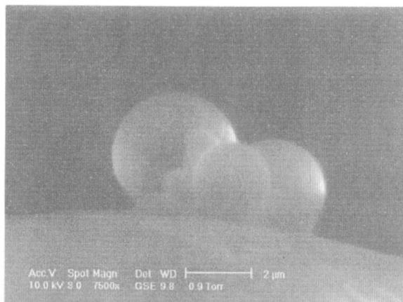
Figure 11: ESEM of polystyrene produced by dispersion polymerization of styrene in SCCO 2 with PS- b -PMPS as the surfactant.
